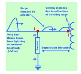
Figure 2 Separation Distance Calculator Circuit
