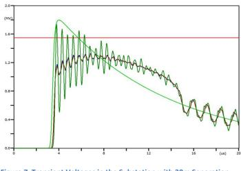
Figure 7 Transient Voltages in the Substation with 30m Separation Distance
