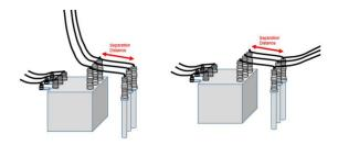
Figure B1 Arrester/Transformer Configurations with arrester before and after transformer
