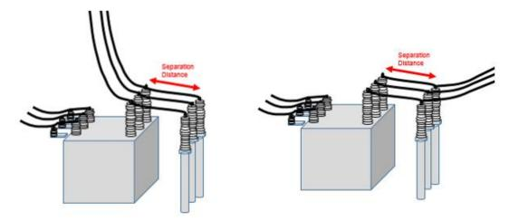
Figure 8 Configurations that are electrically the same and have the same effect on the Transformer Voltage
