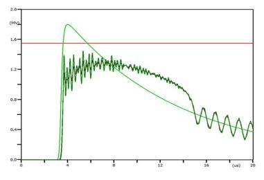
Figure 6 Transient Voltages in the Substation with 15m Separation Distance
