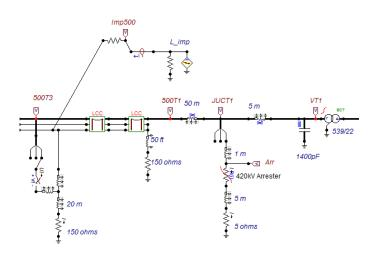
Figure 4 Circuit Modeled in ATP
